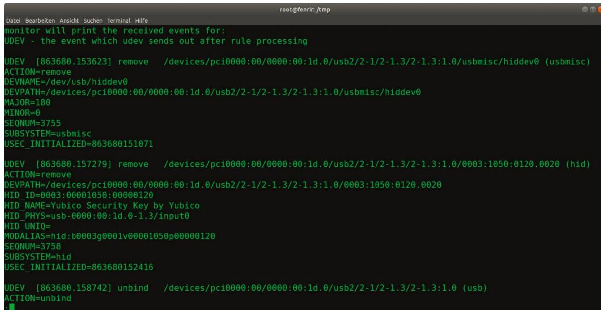
The screenshot shows a terminal window titled "root@fenrir:/tmp". The window displays the output of a command that monitors udev events. The log entries show the removal of three devices: a USBmisc hiddev0 (YubiKey), a hid device (Yubico Security Key by Yubico), and a standard USB device. Each entry includes details like ACTION=remove, DEVNAME=/dev/usb/hiddev0, and various ID and PHYS values.
